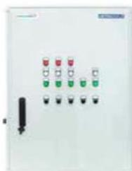
Control and power devices for up to 3 pump sets with soft start devices and control for the compensation tank. The panel includes analog inputs, control of motorized valves in the suction battery and lighting control devices.
